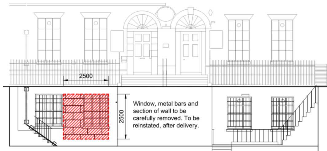
Fig 4. Proposed front elevation (basement level) showing area of demolition in order to install cancer treatment machinery.
