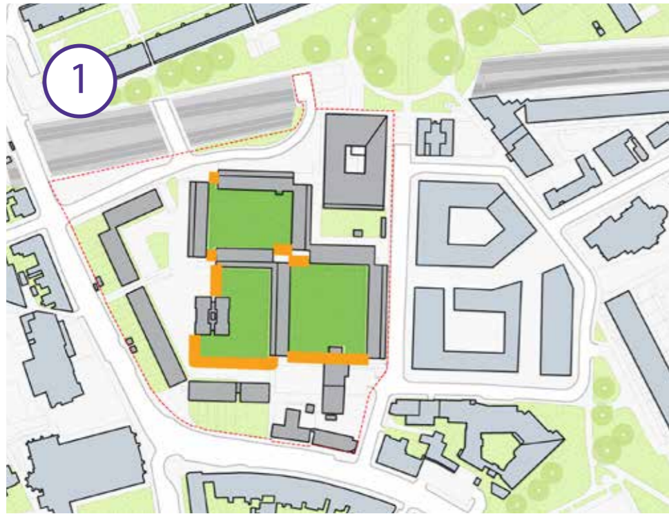
1 LACK OF ACTIVE FRONTAGE
