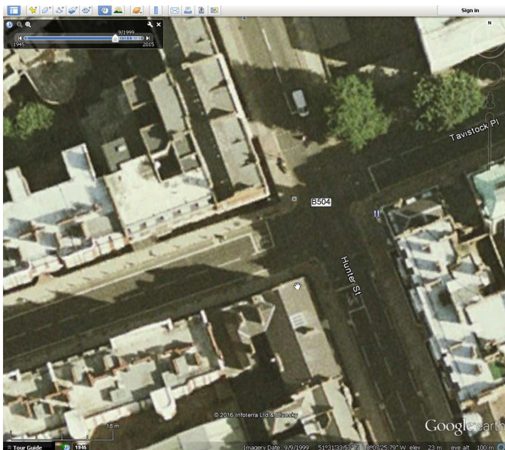
Junction of Tavistock Place and Judd Street/Hunter Street (in 1999), showing two separate cycle lanes, – east- and west-bound, on Tavistock Place.
