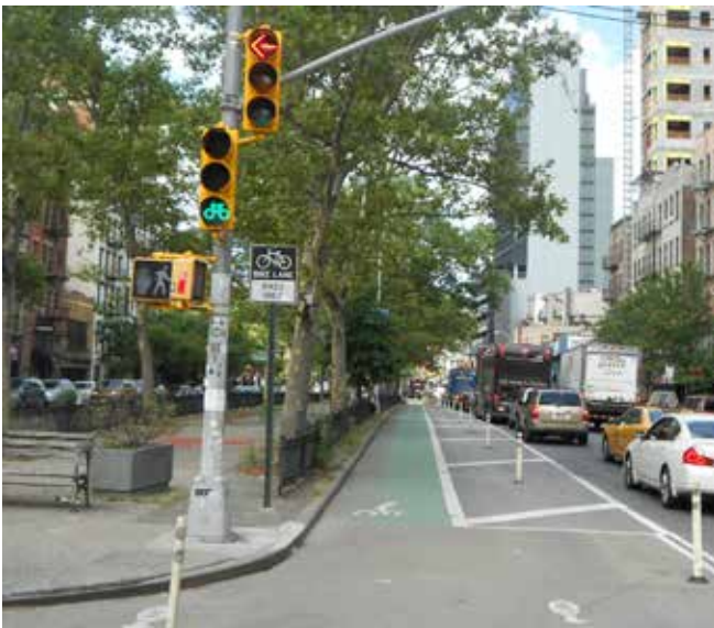
Flexible wands, with extra-wide painted buffer strip: New York
