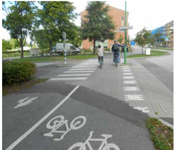
Unsignalised crossing of a side street in Malmo, with cycle track immediately alongside pedestrian path
