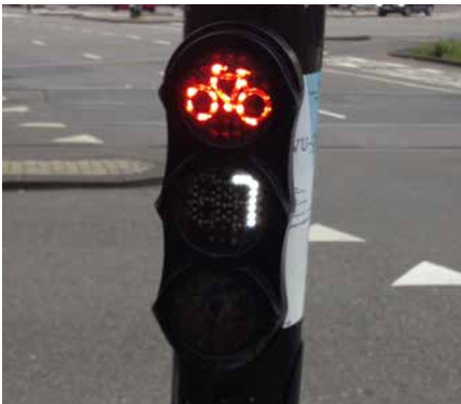
Amsterdam - low level cycle signal with 'count up' (to next green)
