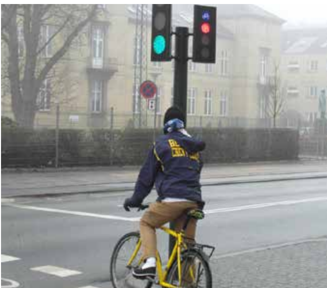
Copenhagen - high level cycle-specific signal aspect
