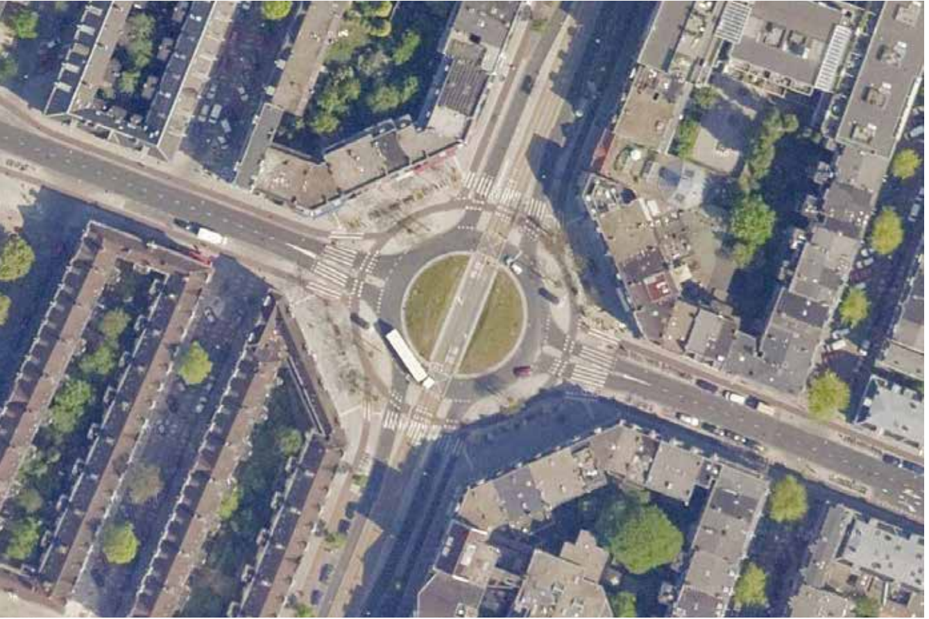
Aerial view from Google of the 'Type 6' roundabout in Amsterdam (see also bottom left picture on page 62). Tram tracks run north-south through the junction.
