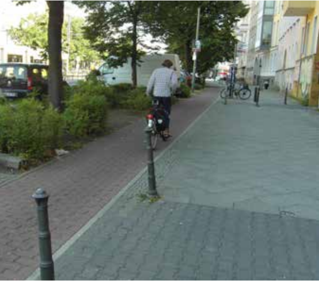
Berlin: different colours, materials and patterns used to distinguish cycle path from adjacent footpath
