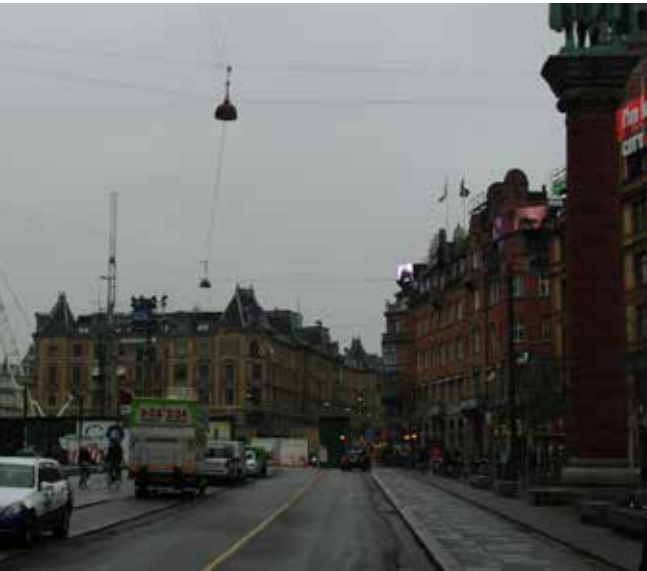
Copenhagen - suspended street lights minimise the numbers of poles at surface level...
