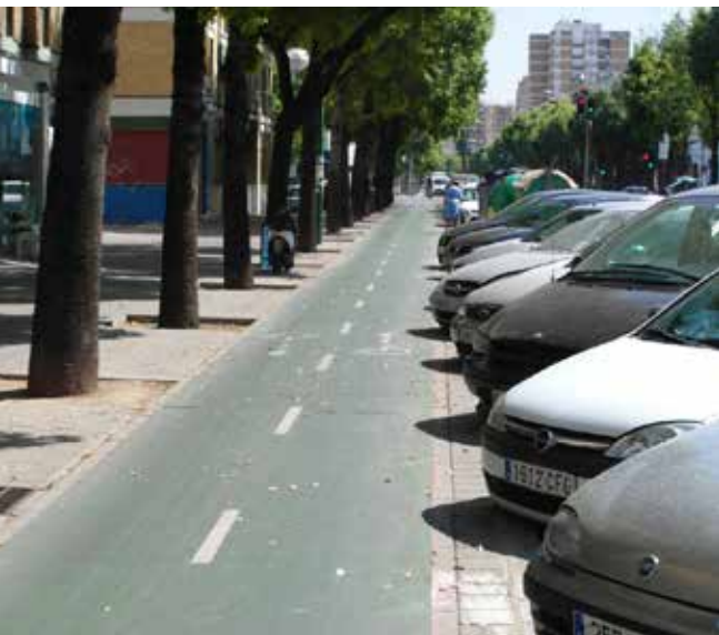
Seville - cycle track replaced car parking. Angled car parking (more spaces) now occupies what was a running lane
