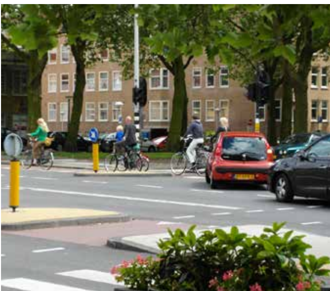
Amsterdam - right-turning car drivers giving way to cyclists going ahead while both have a green signal
