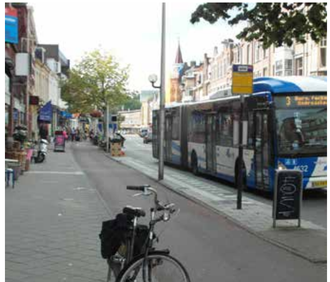
A very narrow 'floating' bus stop in Utrecht, though passenger demand in this location is low.
