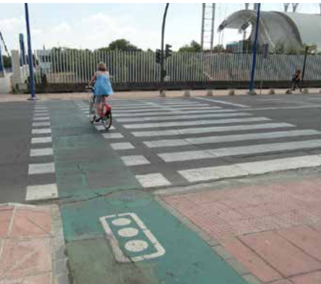
Parallel crossings on one arm of a signalised junction in Seville
