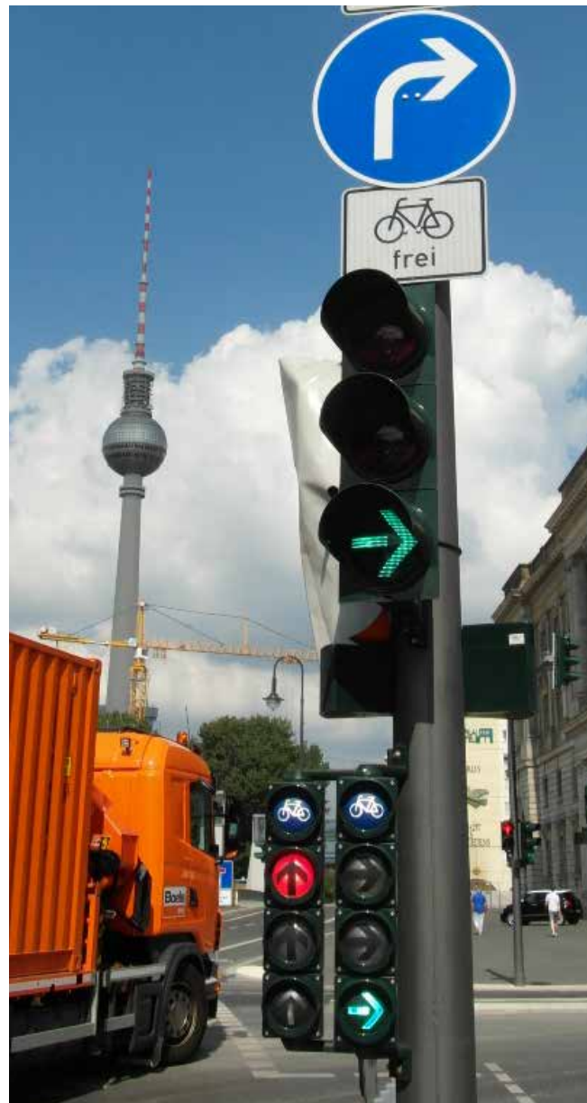
Berlin - distinct sets of low-level cycle signals controlling different manoeuvres
