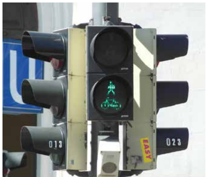
Joint pedestrian-cycle signal at a parallel crossing in Munich
