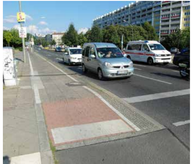
Berlin - stepped cycle track extended in advance of general stop-line
