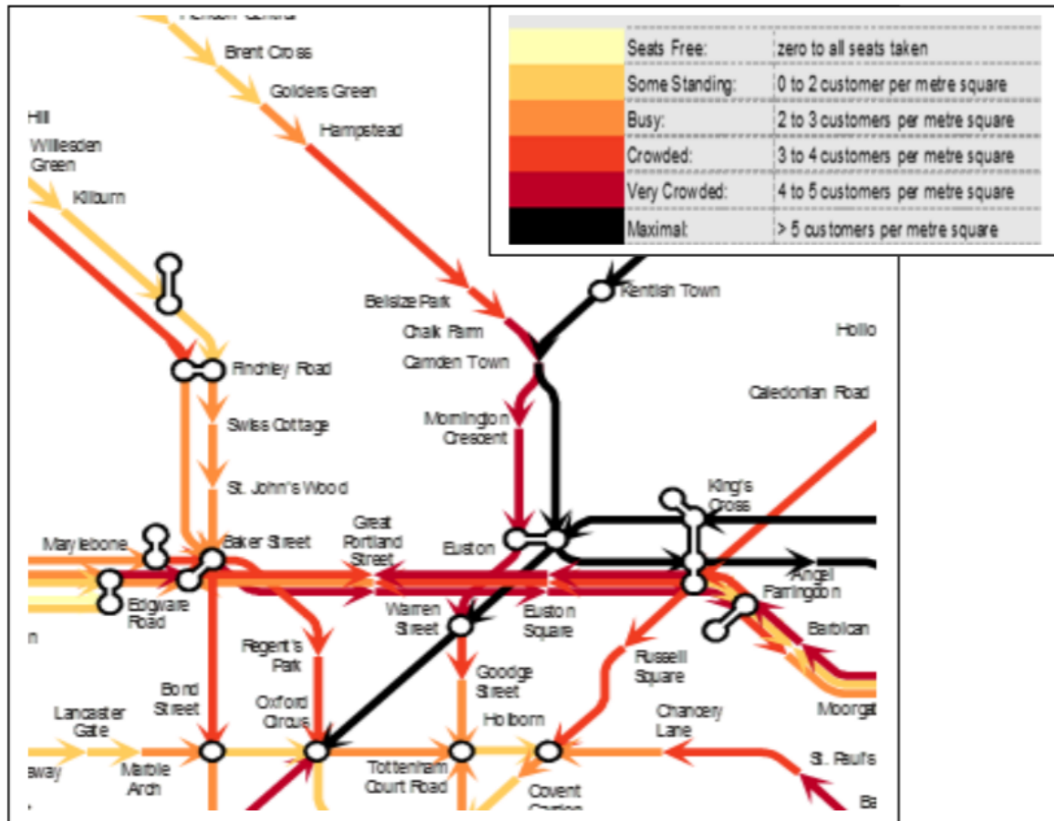
Figure 3 Tube network overcrowding in Camden by 2031 (weekday peak AM hour, includes planning investment) 14
